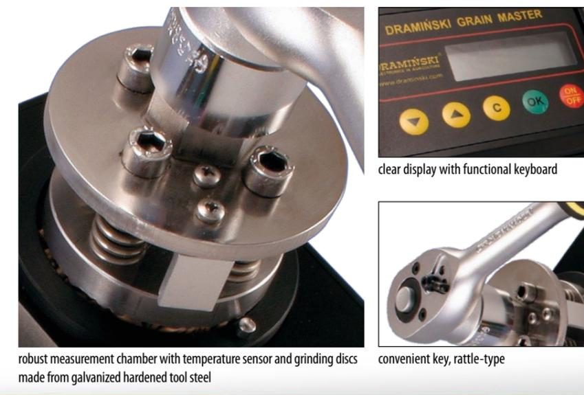
robust measurement chamber with temperature sensor and grinding discs made from galvanized hardened tool steel
